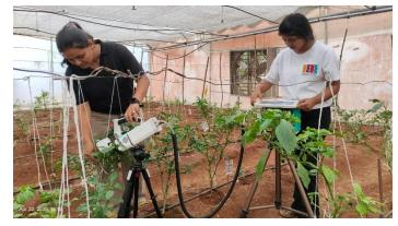
farming. For this, a polyhouse structure of 390 ft<sup>2</sup> (30 ft long \*13 ft width) was constructed at Pabal campus with fan-pad and fogger system. Data on total heat-capture, cooling efficiency of 3 different types of foggers and evaporative pad was collected by using automated temperature & humidity sensors. This data will be useful for development of low-cost, energy-efficient climate control system for farmers.
